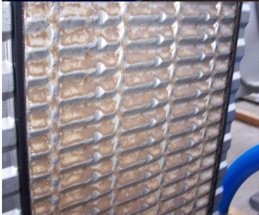
Plate heat exchanger with 12mm plate spacing
